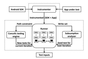
Figure 8: Dataflow diagram of our system.
